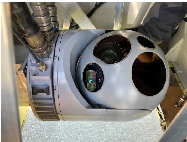
Figure A3.1. Aerial surveys in Southeast Alaska (excluding Glacier Bay) were flown in the Owyhee Air Research P68C. Two camera sensors were attached to the aircraft: an L3/Harris MX-10 IR/RGB video system (bottom left) in the belly port and a Waldo XCam Ultra 50 (bottom right) under the front passenger seat.
